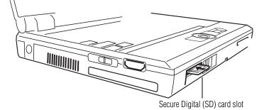
Sample inserting an SD card
